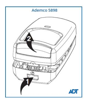
4. Remove the old battery. You may need to use the flathead screwdriver to gently lift the battery from the device. Some devices may have two or more batteries. If this is the case, make sure you remove and replace all batteries at the same time.
